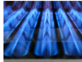
Combustion experiment using 20% hydrogen mixed gas
