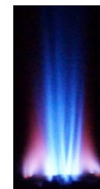
Combustion experiment with 100% hydrogen (small amount of methane mixed with hydrogen since hydrogen is not visible)
