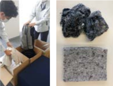
Uniforms being collected Cotton-like state after crushing
