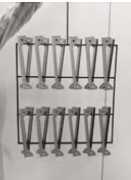
Painting line: Hob (stovetop) parts being hung (Oguchi Factory)
