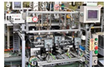
Inspection of the entire number of temperature sensors on the assembly line of gas stoves
