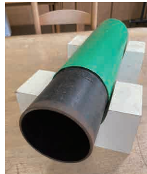
Hydrogen piping (installed underground)
