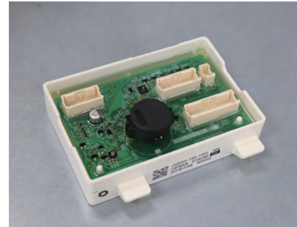
Control board for a gas stove containing an earthquake detection program
