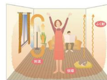
Three Advantages: radiance, conduction, and convection
