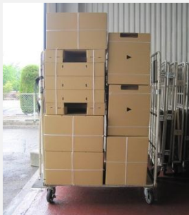
Cartons are fixed to each other with plastic string Number of cartons loaded on wheeled platform: 20
