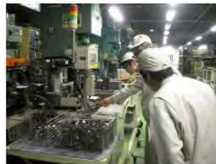
Workers make the rounds and check for air leakages.
