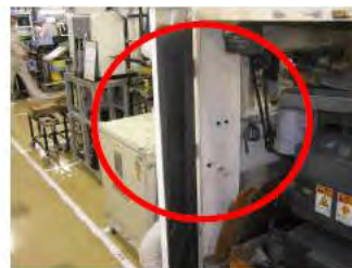
Heat insulating materials to prevent losses resulting from heat dissipation
