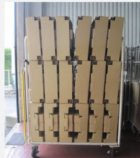
Plastic string eliminated Number of cartons loaded on wheeled platform: 36
