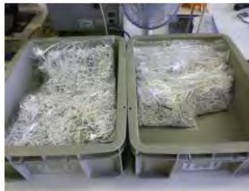
Cushioning materials made from shredded sheets of paper
