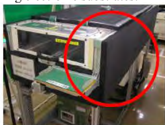
Heat insulating materials to prevent losses resulting from heat dissipation
